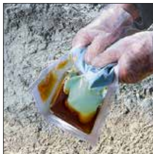
The middle cold seal between the resin and hardener component opens by means of pressure.
